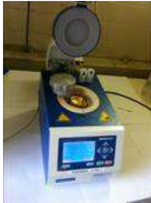
Figure 1 - Photography of Apparatus for Rapid Small Scale Oxidation Test
