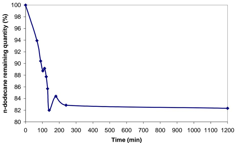
Figure 5 – Consumption of the n-dodecane during the test
