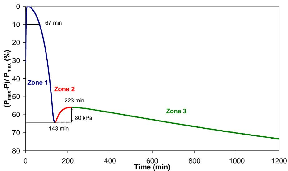
Figure 4 – Evolution of normalized pressure drop versus time
