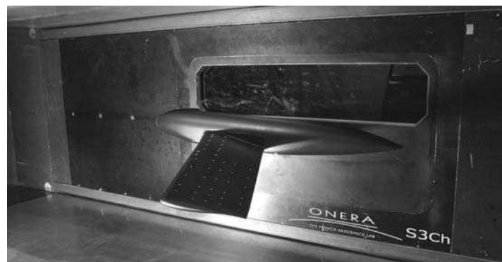
Figure 1 - Experimental set-up in the S3Ch wind tunnel.
