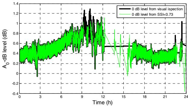
Fig. 4.  $A_0$ -dB level for the beacon measurements on December 7, 2012, using as threshold (top)  $SSI < 0.87$  and (bottom)  $SSI < 0.73$  as compared with CPA derived from visual inspection (black curve).
