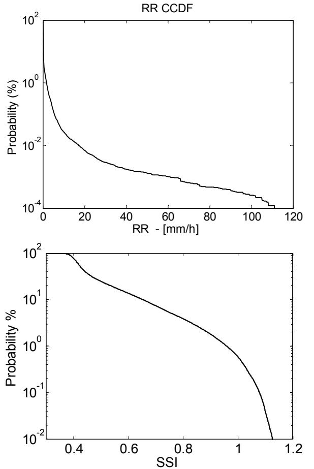
Fig. 1. (top) CCDF of  $RR$  derived from the pluviometer measurements collected at Onera between July 2012 and June 2013. (Bottom) CCDF od  $SSI$  derived from the ground-based microwave radiometer.
