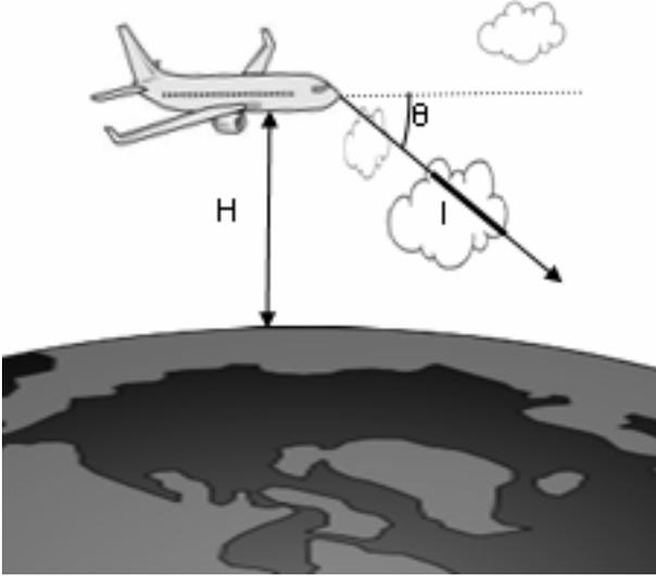
Figure 2. Viewing geometry of an airborne sensor at height  $H$ , with viewing angle  $\theta$ .  $l$  is the segment of the sensor LOS crossing the cloud layer.
