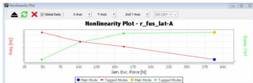
Fig. 15 : Linearity plot (resonance frequency and structural damping ratio / Generalized excitation Force)
