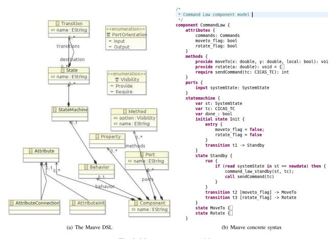
Fig. 2: Mauve component model
