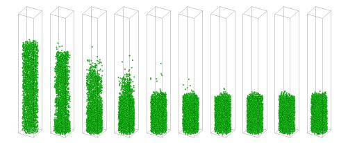
Figure 1: Three-dimensional view of the particles inside the fluidized bed from left to right, t = 1, 2, 3, 4, 5, 6, 7, 8, 9 and 10s.
