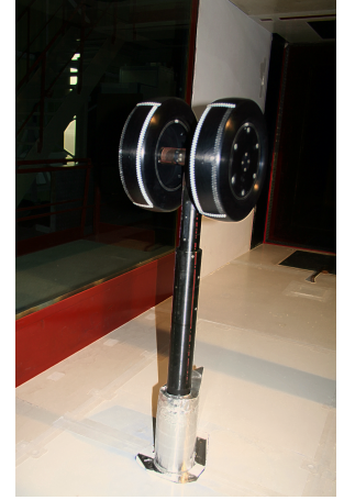
Figure 1. LAGOON baseline configuration. Main dimensions (left) and F2 wind tunnel setup (right)
