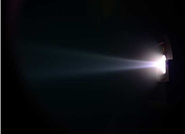
Figure 4 – Typical plasma plume produced by ECR source
