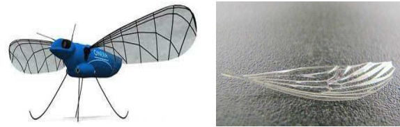
Figure 11: ONERA microdrone Remanta and wing prototype obtained by stereo photolithography
