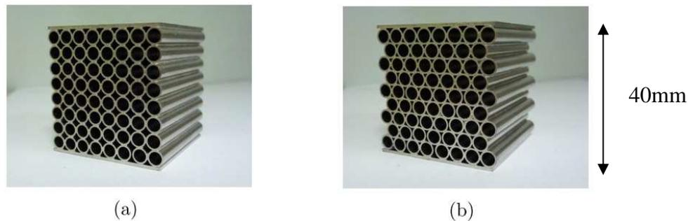
Figure 1: Arrangement of hollow tubes for fabricating cellular structure (a) square and (b) hexagonal stacking.
