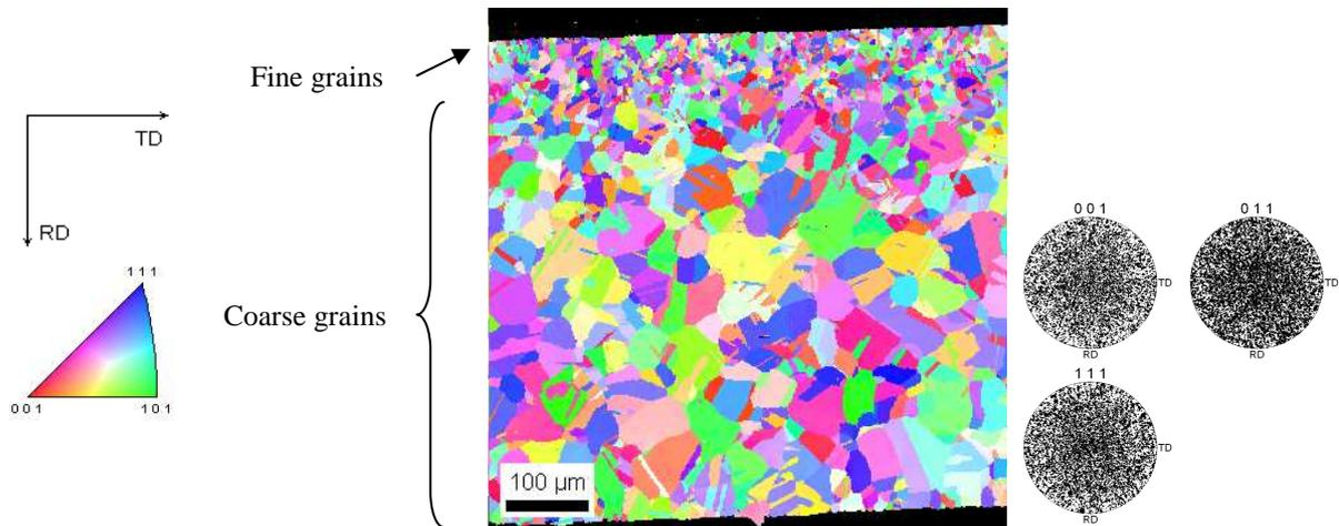
Figure 7: EBSD analysis of a Inco600BM tubular specimen in a non-loaded Inco600BM tubular specimen in the central area: Orientation mapping referring to TD axis direction and key color; the corresponding pole figure.
