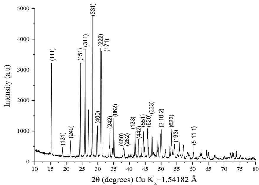
**Figure 2 - XRD pattern of AgGaGeS<sub>4</sub> polycrystalline sample**
