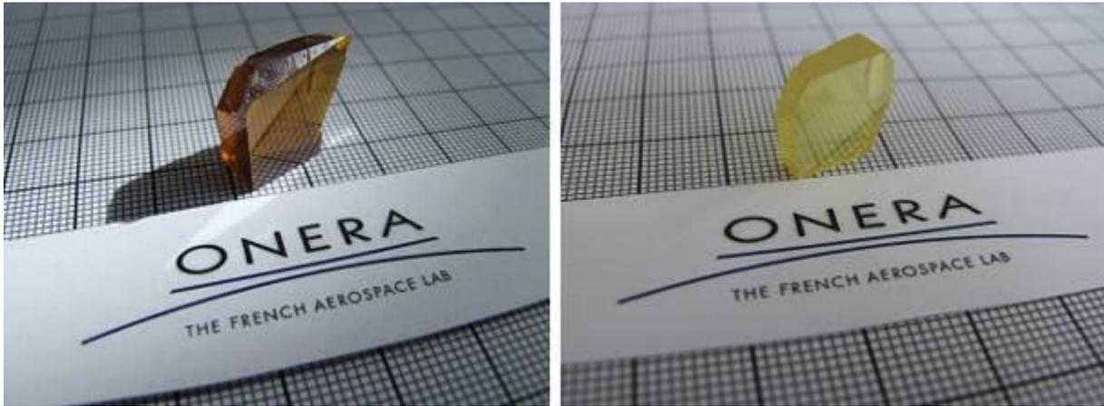
**Figure 3 - Picture of a polished as-grown (left) and post-treated (right) AgGaGeS<sub>4</sub> single crystal.**
