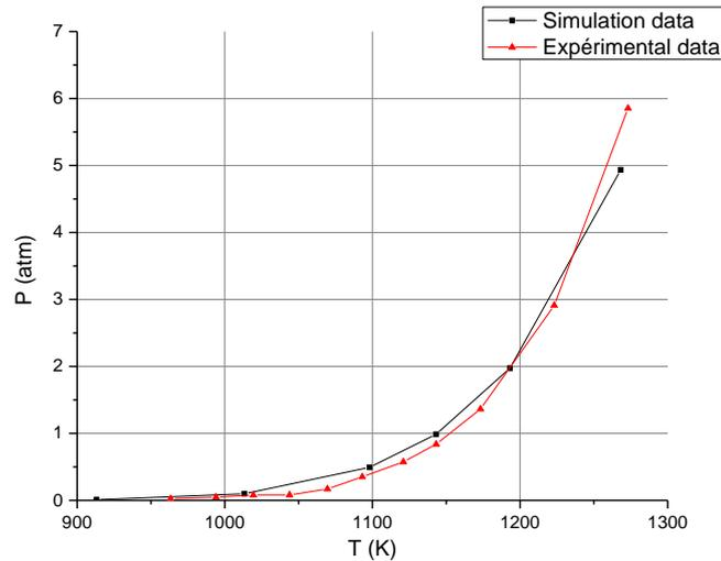
**Figure 4 - Plot of calculated GeS<sub>2</sub> vapor pressure versus temperature and experimental data from ref [5].**
