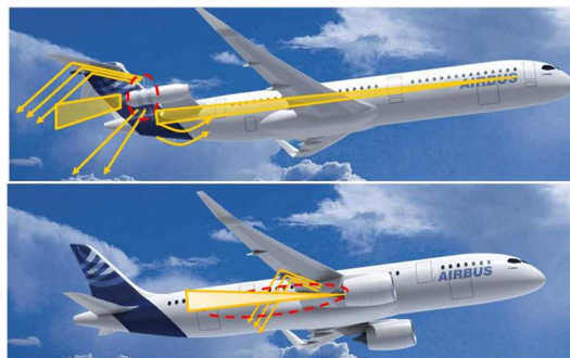
Figure 13. Noise emission and acoustic installation effects of CROR- and HBPR- engines powered aircraft, to be numerically assessed in EC projects JERONIMO and NINHA, respectively (Airbus courtesy).
