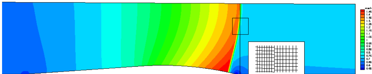
Figure 10. Delery nozzle, Mach number contours.
