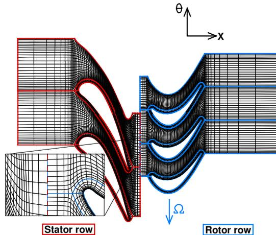
Figure 1. Example of rotor/stator configuration and blow-up of the patched grid at rotor/stator interface.
