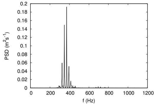
Figure 2: PSD of a laminar velocity signal
