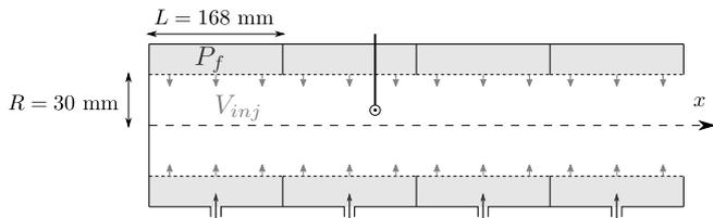
Figure 1: Geometry of the VALDO setup
