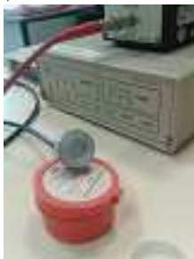
Figure 9 – Bancal system (PIN diode detector)
