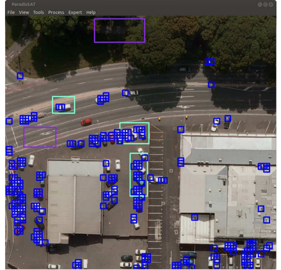
Fig. 7. Result of the interactive learning process of Fig. 1 with detections of cars (blue squares) on an orthorectified aerial image of resolution 0.1m.
