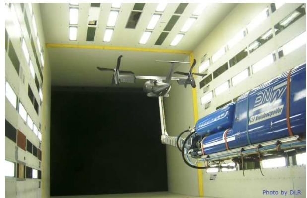
Figure 1: Conversion configuration in the DNW-LLF wind tunnel.
