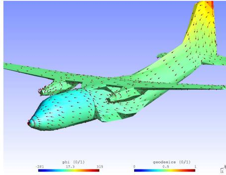
Fig. 2 Global lightning current from rear to nose.
