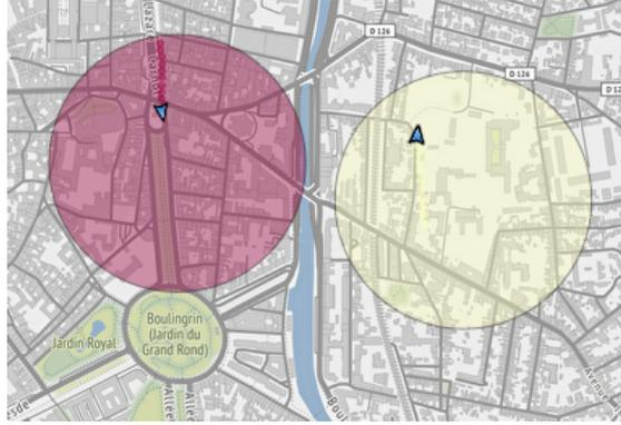
**Fig. 2 4D protection bubbles around drones.**
